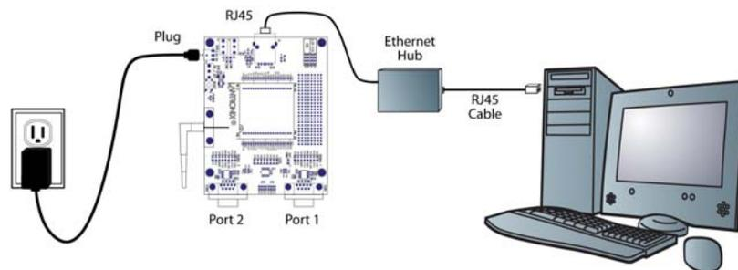
2. Select the appropriate power plug adaptor for your geographical location. Insert it into the slot on the Universal Power Supply; then plug the power supply into an outlet.
