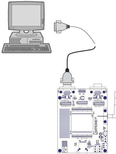
In the event that the equipment required for a network connection is not available for the initial configuration of the MatchPort, the serial method can be used.
