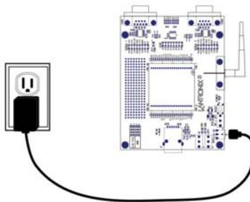
3. Select the appropriate power plug adaptor for your geographical location. Insert it into the slot on the Universal Power Supply; then plug the power supply into an outlet.
