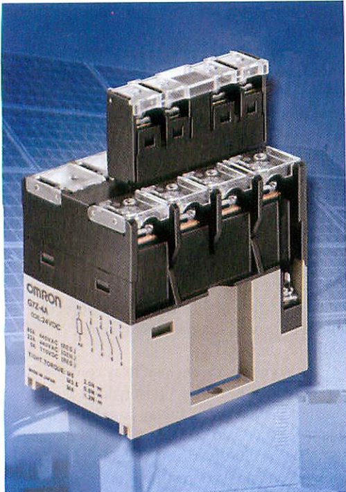
A heavy-duty power relay switches power in solar-battery and motor-control applications and in uninterruptible power supplies. This G7Z relay provides four form-A contacts. Courtesy of Omron.
