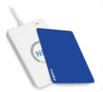
The ACR122 is a PC-linked Contacless Smart Card Reader/Writer developed on the 13.56MHz Contactless Technology. It is the world's first CCID Compliant Contactless Card Reader/Writer that follows both ISO14443 and ISO18092. This device is designed to support not only MiFare and ISO14443 Type A and B Cards but also FeliCa and NFC tags.
